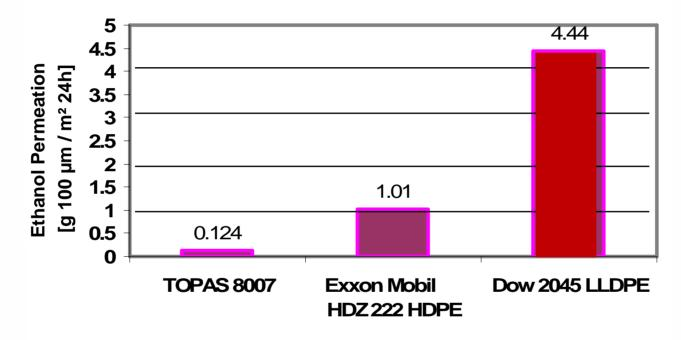
COC has significantly reduced ethanol permeability as compared to other polyolefins\*.
