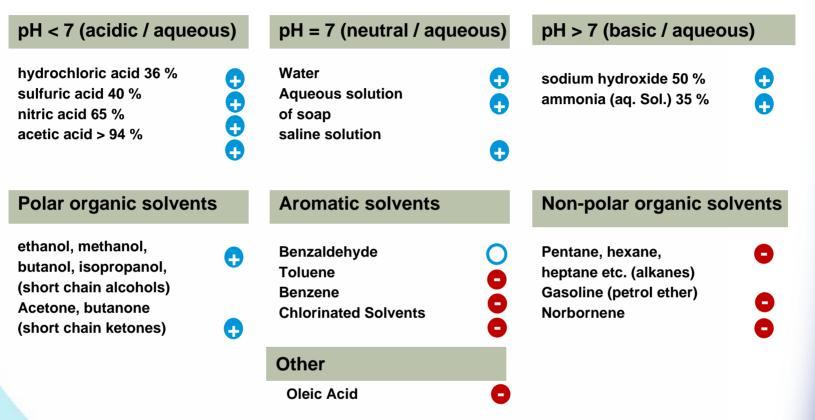
es resistant, increase of weight < 3% or loss of weight < 0,5%, elongation at break not substantially altered
