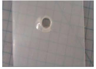
85% 8007 15% Elastomer 470 lb<sub>f</sub> 22.3 ft-lb 85% 9506 15% Elastomer 474 lb<sub>f</sub> 22.9 ft-lb 40% 9903D-10 40% 6013M-07 20% Elastomer 436 lb<sub>f</sub> 19.8 ft-lb
