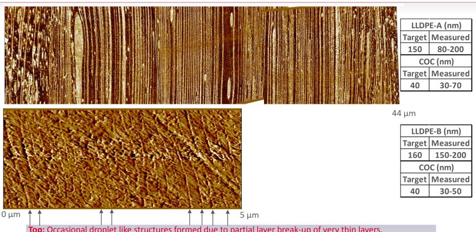
Top: Occasional droplet like structures formed due to partial layer break-up of very thin layers.
