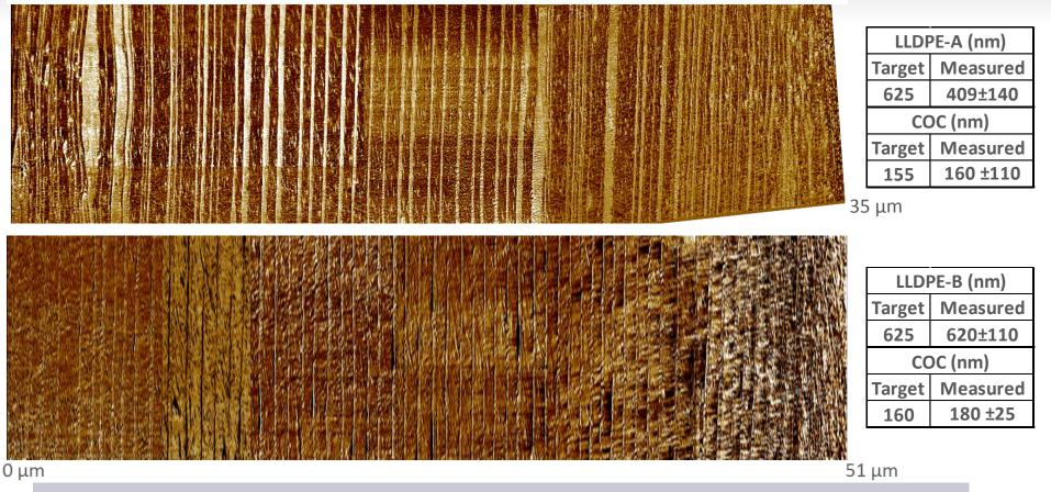
**Top**: 5 μm section on each side of the film was not imaged. 40+ distinct layers of COC and 40+ distinct layers of LLDPE could be seen in the imaged section. Layer integrity appears better in the middle layers.
