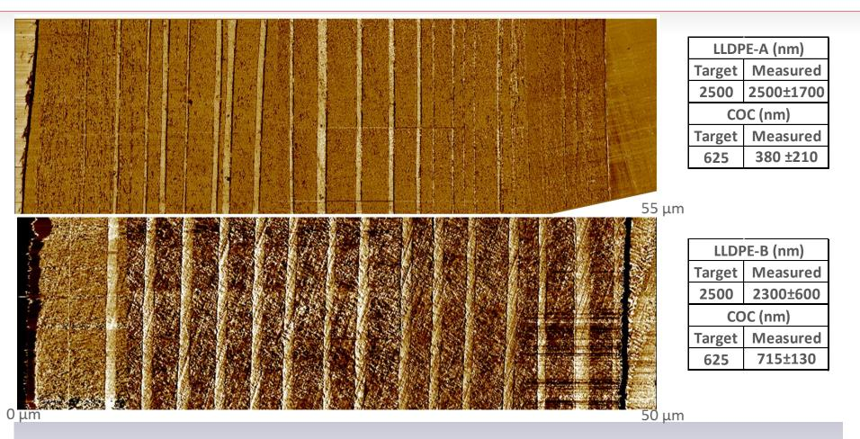
Rheological property difference between LLDPE-A & COC at processing temperatures led to layer thickness variation. With exception of both outermost COC layers; considerably less layer thickness variation observed for LLDPE-B / COC.
