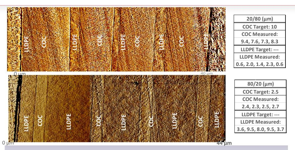
Both films have good layer stability and minimal layer thickness variation. Measured layer ratios are 19/81 and 78/22 respectively, close to targets.
