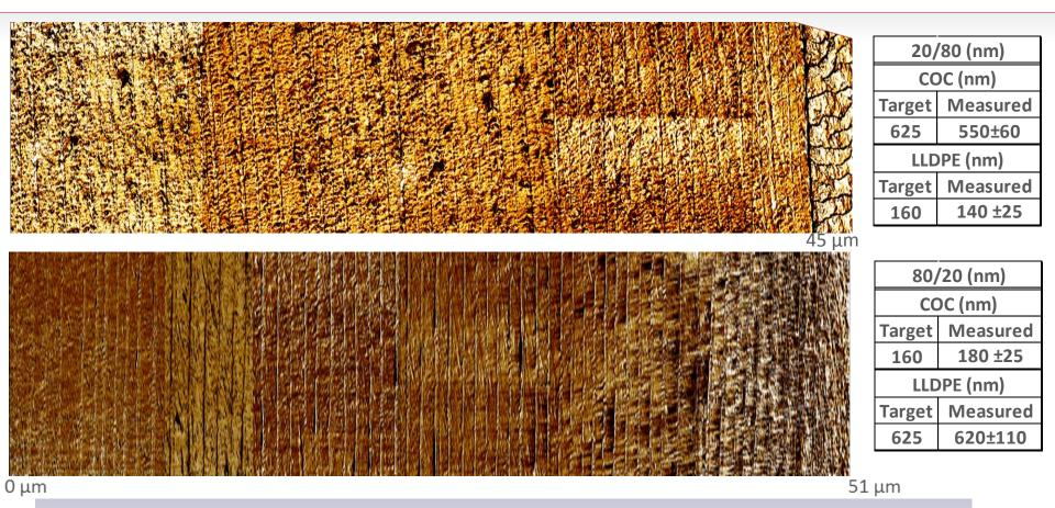
Top: 126+ layers were imaged. Leftmost layer could not be imaged due to significant delamination between epoxy-LLDPE interface. Overall, the film showed good layer structure and periodicity. No layer break-up was observed.
