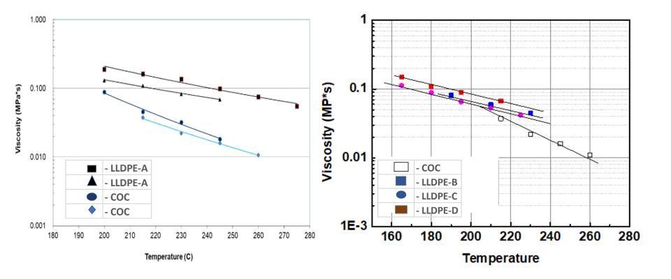
LLDPE-B shows closer viscosity match to COC than LLDPE-A. Process temperatures in layer replicating units were 200 - 210°C.
