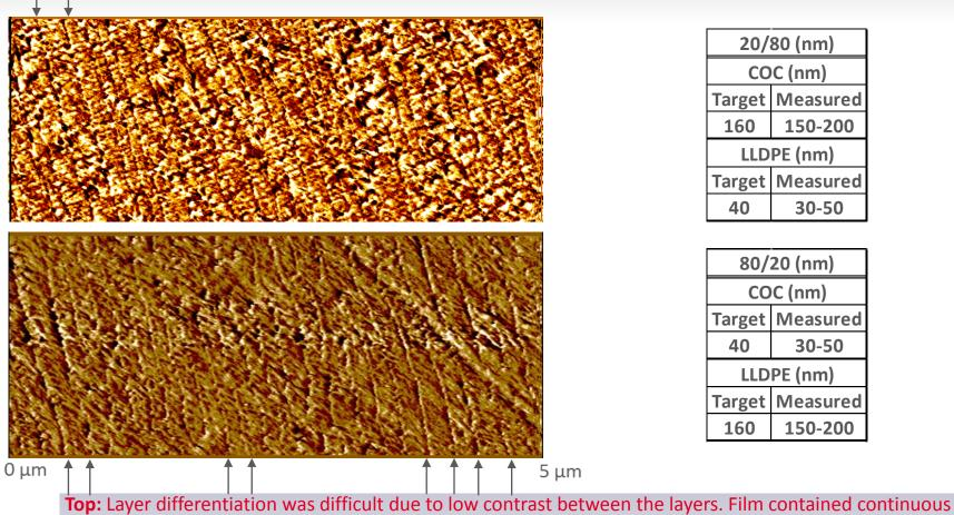
layer in the imaged section. Black arrows represent 30-50 nm LLDPE layers. **Bottom**: Film contained continuous layers, with possible partial layer break-up. Dark arrows represent 30-50 nm COC layers.
