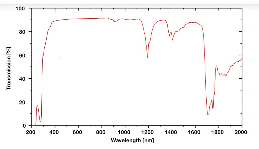
The high transparency of TOPAS in the visible and near ultraviolet range is attractive for optical components
