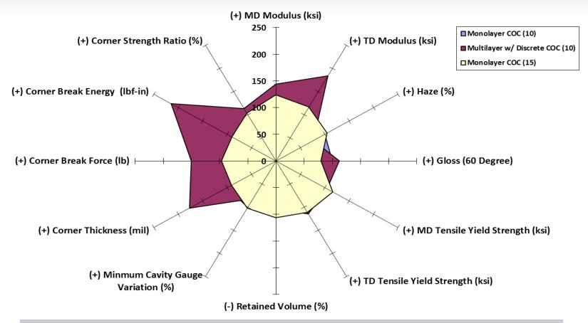
10% COC discrete layer construction offers <u>cost savings</u> improvement to many properties vs. 10% & 15% monolayer blend Best enhancements: Modulus, and Formed Cavity Corner Puncture
