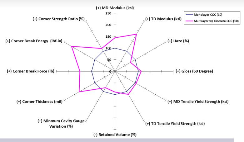
10% COC discrete layer construction offers "free" improvement to many properties vs. 10% monolayer blend
