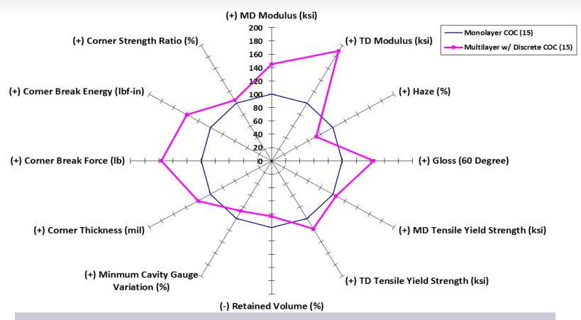
15% COC discrete layer construction offers "free" improvement to many properties vs. 15% monolayer blend
