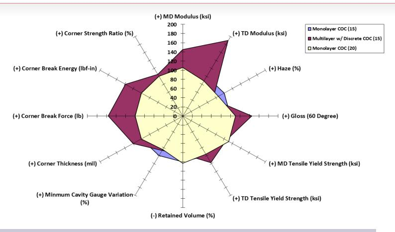
15% COC discrete layer construction offers <u>cost savings</u> improvement to most properties vs. 15% & 20% monolayer blend Best enhancements: Modulus, and Formed Cavity Corner Puncture
