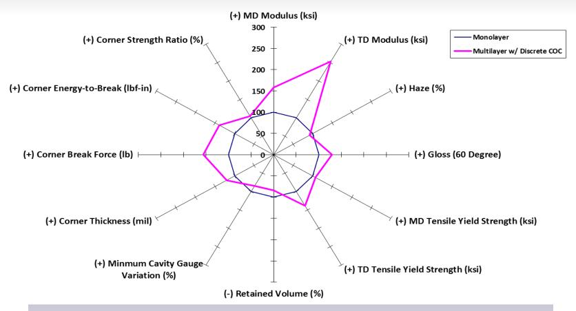
20% COC discrete layer construction offers "free" improvement to many properties vs. 20% monolayer blend
