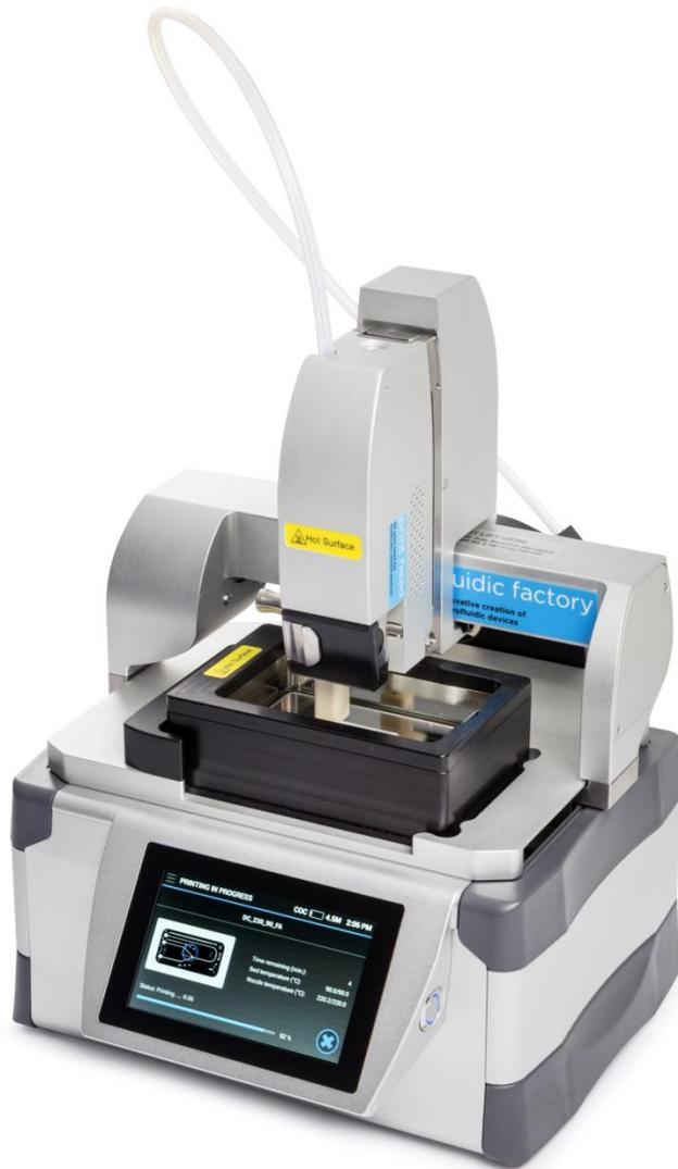
Dolomite, based in the U.K., recently launched the Fluidic Factory, the first commercially available 3D printer for fluidically-sealed devices made of TOPAS 8007S-04 COC.
