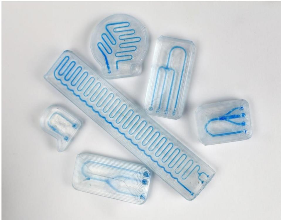
A variety of microfluidic chips are produced on Dolomite's Fluidic Factory, the first commercially available 3D printer for fluidically-sealed devices made of COC.
