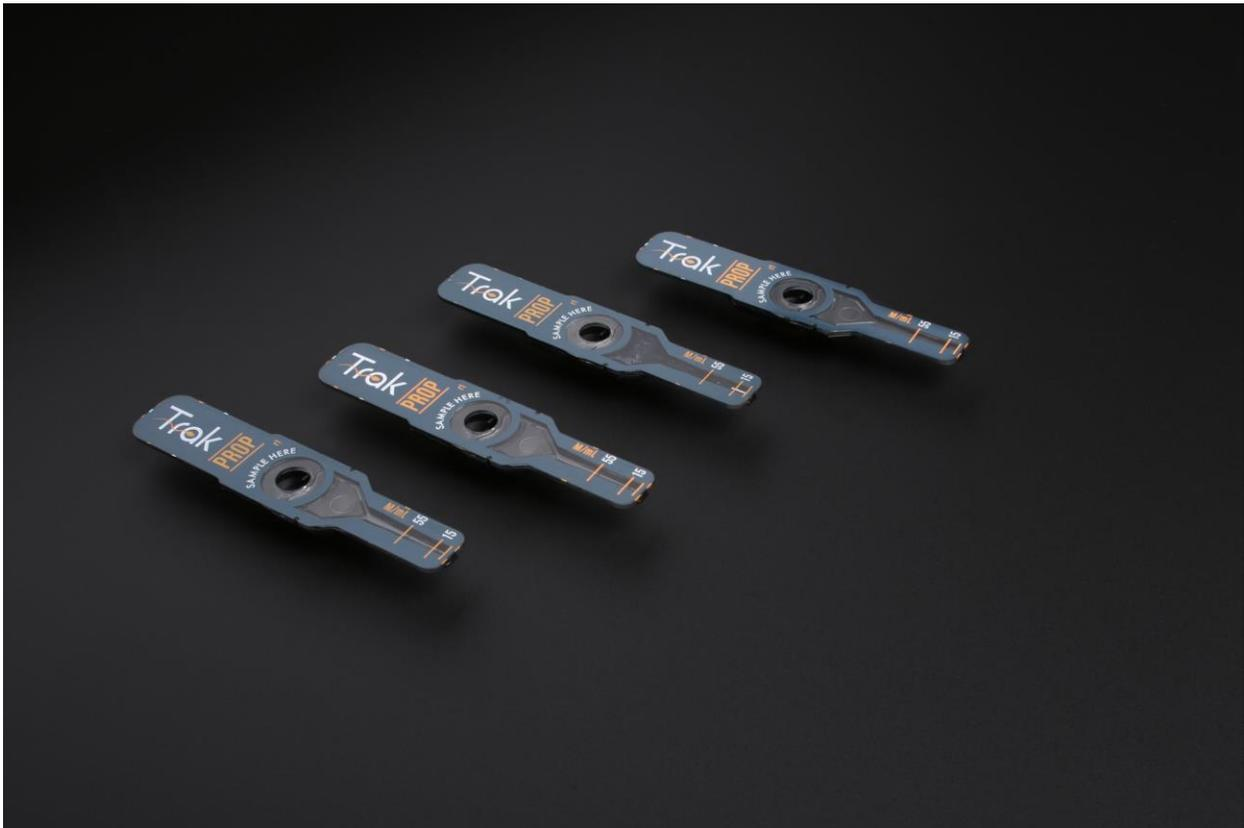
Sandstone Diagnostics' Trak® Male Fertility System is a microfluidic device which uses TOPAS 8007S-04 COC in its disposable cartridge.
